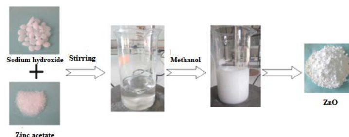
Figure 1. Zinc oxide synthesis steps
