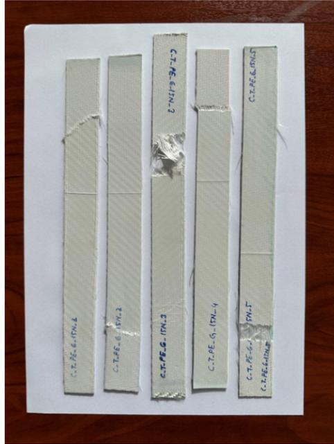
Prestressed and non-prestressed glass fiber fabrics were subjected to three-point bending tests, each with 5 separate specimens with dimensions of 150x12.7x1 mm.
