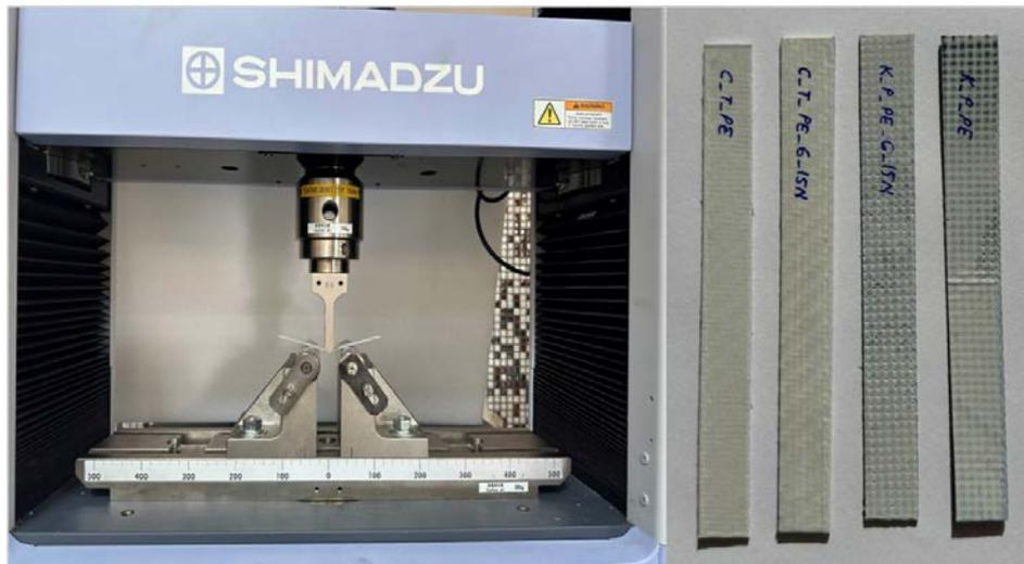
Since there is no stretching in the prestressed materials, the ability to move in the thermoplastic matrix is less, failing the pre-stressed specimens for the three-point bending test.
