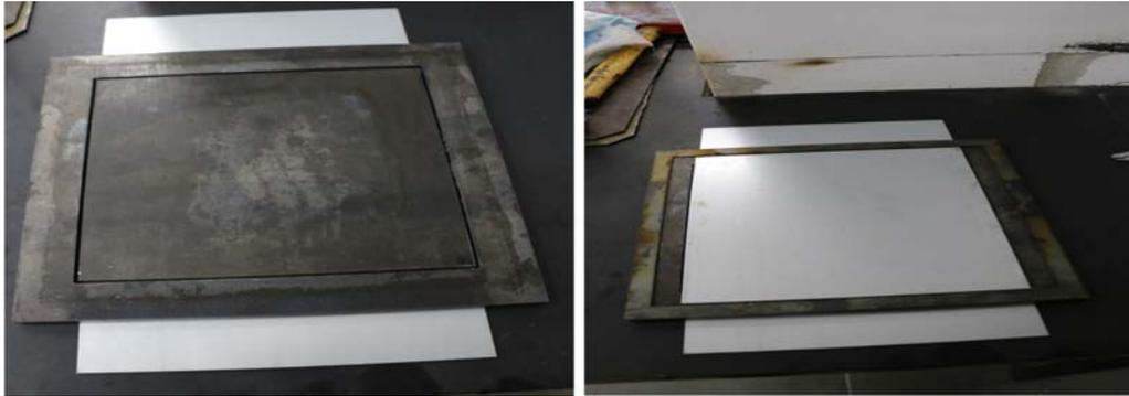
After fabrication, heat-resistant greaseproof paper was used to prevent easy removal of the specimens from the sheet frame and to prevent sticking. The specimens prepared without pre-tensioning were placed in a hydraulic press and cured under temperature and pressure. The temperature was gradually increased by paying attention to the melting temperature of the matrix material PE film and homogeneous distribution of the film layer in the fiber pores was ensured.
