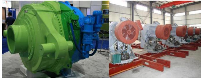
Large turbine (over 1000kW) generators typically produce 3-phase voltage at 690 V, which is then stepped up to 10-30 kV using transformers before being fed into the distribution or interconnected network. Small power generators utilize small blades, while large blades are only efficient in strong winds, where they can generate power close to the generator's capacity, minimizing waste. However, large generators struggle to operate at low wind speeds.
