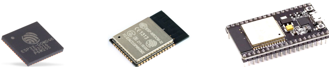
Figure 10. ESP32 SoC, Module (ESP32-WROOM-32) and Development Board (NodeMCU ESP32-S).
