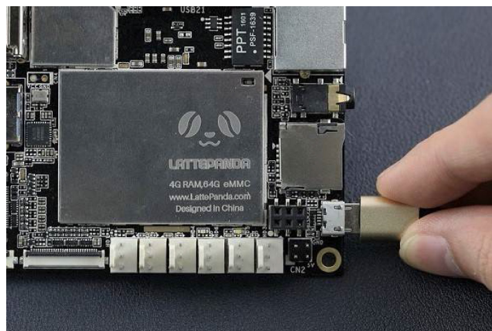
Figure 4. Installing the Display Plug
