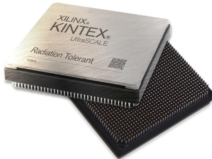
Figure 1. An FPGA IC belongs Xilinx Company
