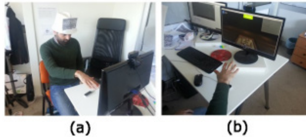
Figure 8. (a) A pointer icon placed on a person's head (marker) and the pointer icon is used to track the camera located on the monitor. (b) The game developed with Leap Motion and the human perspective (Ong et al., 2012).
