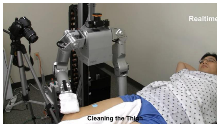
Figure 2. Cody who can autonomously perform the movement of wiping the patient just like a nurse (King, 2010: https://www.youtube.com/watch?v=0ac2qwStrdo ).
