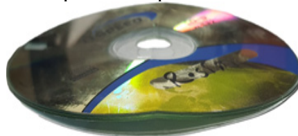
Figure 23. Example of a physically deformed optical disc
