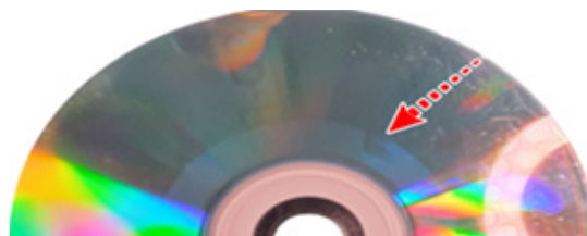
Figure 20. Error during data recording to optical disc
