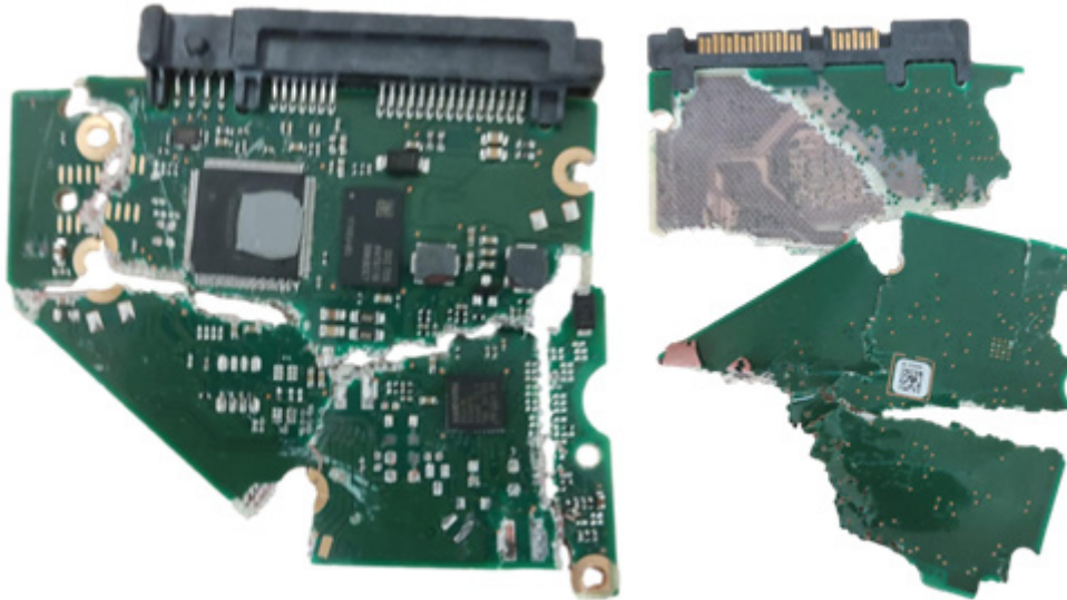
Figure 51. Intentional breakage of the printed circuit board
