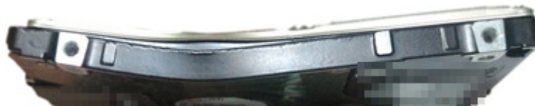
Figure 52. Physical damage to the disk (Recovery HDD, 2018)
