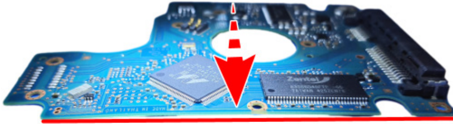
Figure 39. Internal path break in PCB as a result of bending
