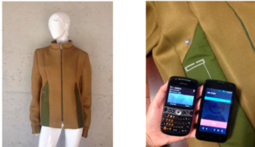
Figure 7. Smart coat with integrated dual band antenna for energy harvesting (Loss et al., 2016)
