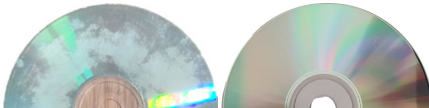
Figure 15. Dirty and cleaned optical disc surface
