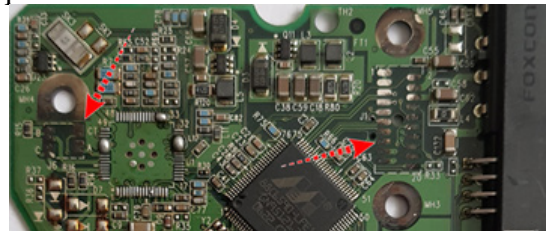
Figure 30. Contamination of pads going to a motor or read/write heads
