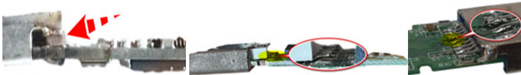
Figure 14. USB socket pins not touching
