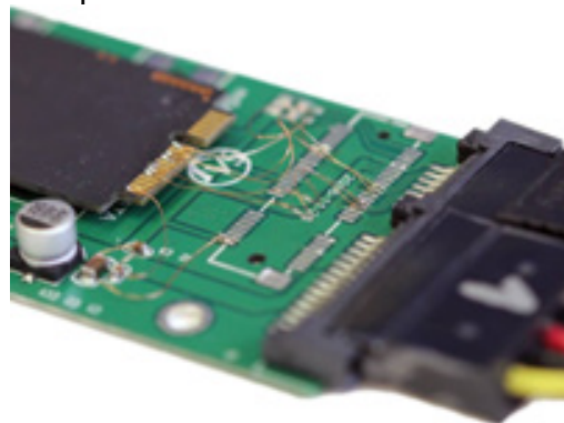
Figure 24. Bus not working after liquid contact with (ITHOPE s.r.o., 2021)
