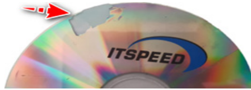
Figure 21. Wear of the reflective surface of the optical disc
