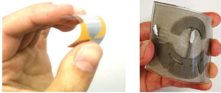
Figure 10. a) Elliptical UWB antenna based on Kapton polyimide material (H. R. Khaleel et al., 2012), b) PDMS-embedded conductive fabric antenna (Simorangkir et al., 2018)
