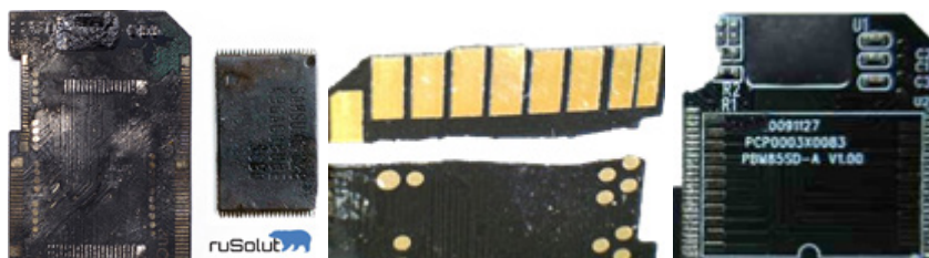
Figure 34. Burnt memory card (Rusolut Sp. z o.o., 2014) and memory cards with broken PCB
