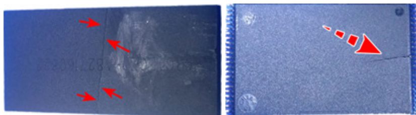
Figure 37. Broken UFD and Tsop48 chip examples
