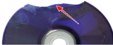
Figure 17. Fracture of the optic disc
