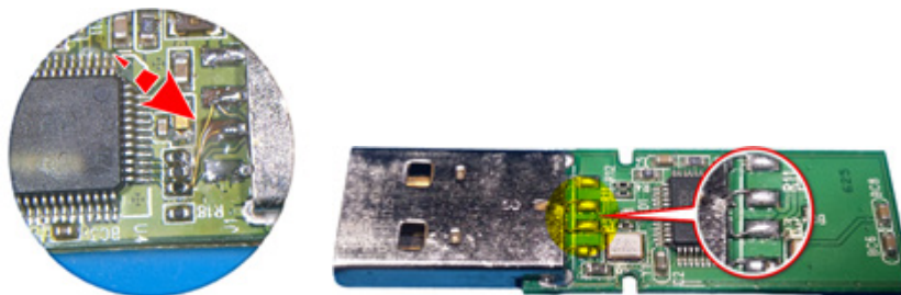
Figure 10. USB bus break
