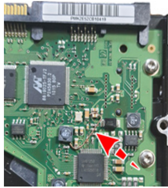
Figure 48. Presence of materials that will block the electric current in the PCB
