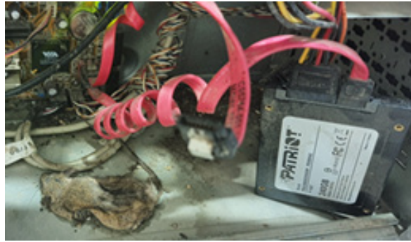
Figure 25. Example of a mouse biting the power cord
