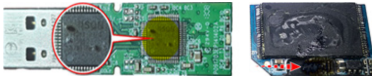
Figure 32. USB flash drive and memory card with damaged controller
