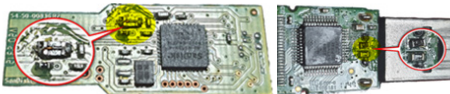
Figure 15. Bad fuse resistor
