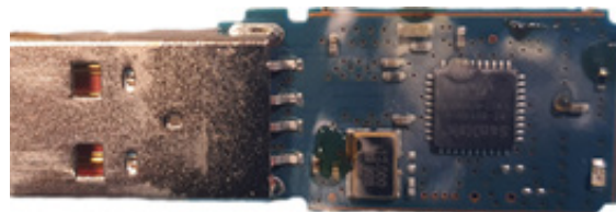
Figure 33. Oxidized USB flash drive
