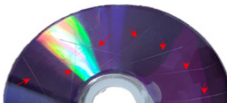
Figure 19. Having deep scratches on the optical disc
