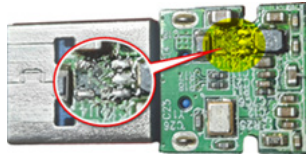
Figure 12. Fragmentation/loss of circuit element
