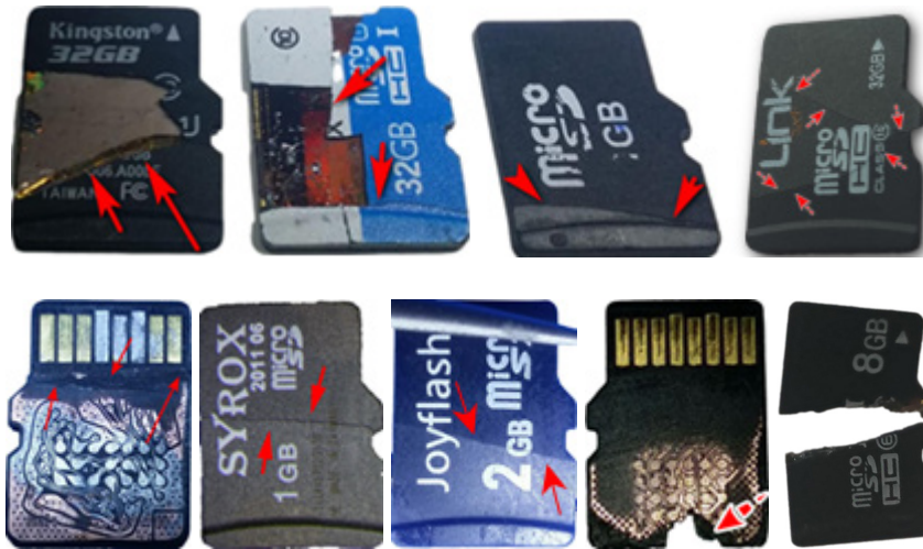
Figure 36. Examples of broken, cracked, and dented memory cards
