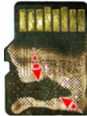
Figure 35. Excessive scraping of the memory card surface
