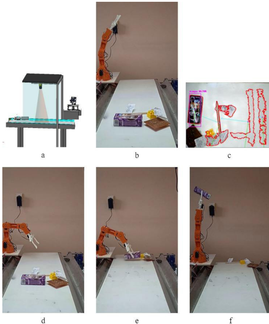
Figure 3. a) General view of robotic vision & grasping mechanism, b) Robot arm and objects to be separated, c) Viewing objects and obtaining deep network related data, d) Positioning of the robot arm according to the deep learning result, e) The robot arm grasps the desired object, f) Separation of the grasped object
