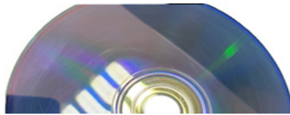
Figure 18. There are light scratches on the optical media
