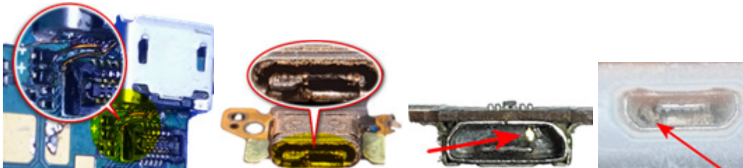
Figure 26. Socket failures in mobile devices
