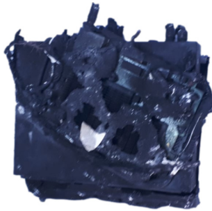
Figure 46. Hdd inside burnt DVR device
