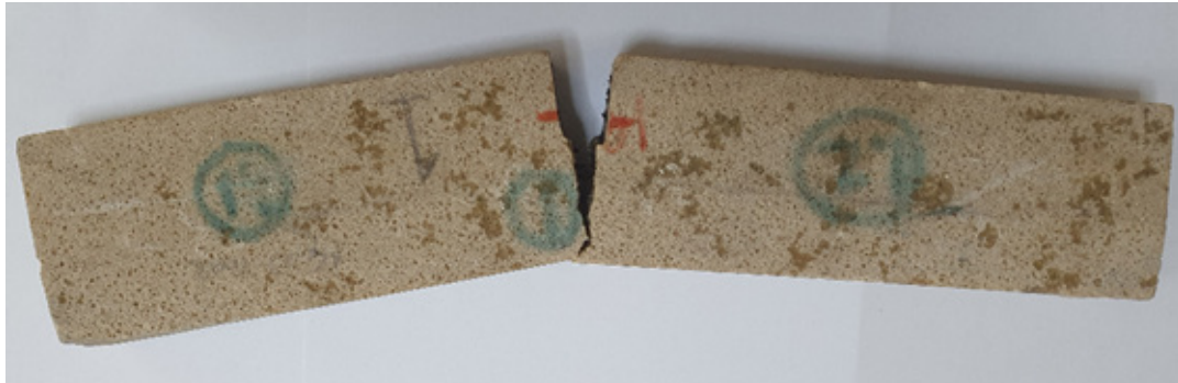
Figure 5. Notched Aggregate Filled Reinforced Polymer Composite Specimen (After Three-Point Bending Test)
