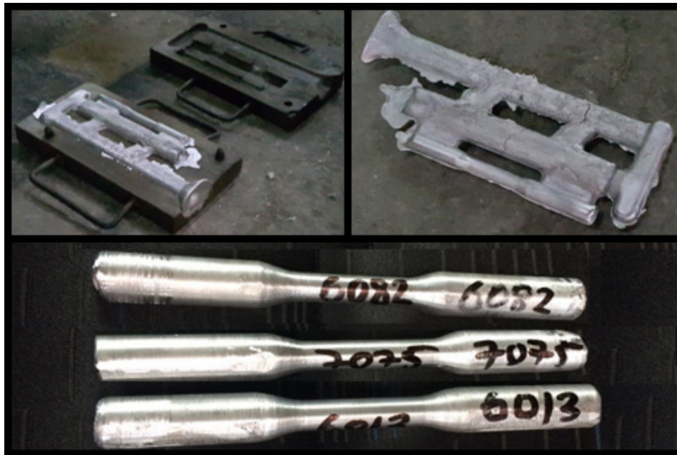
Figure 2. Metallic mould and tensile test specimens
